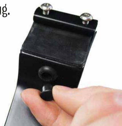
6. Place the luggage rack on the boot-lid and tighten the side brackets.
