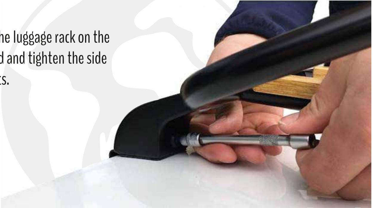
7. Use the supplied two screws on every bracket for extra security. Don't tighten these screws with too much force because they can go through the protective 3-M foil.
