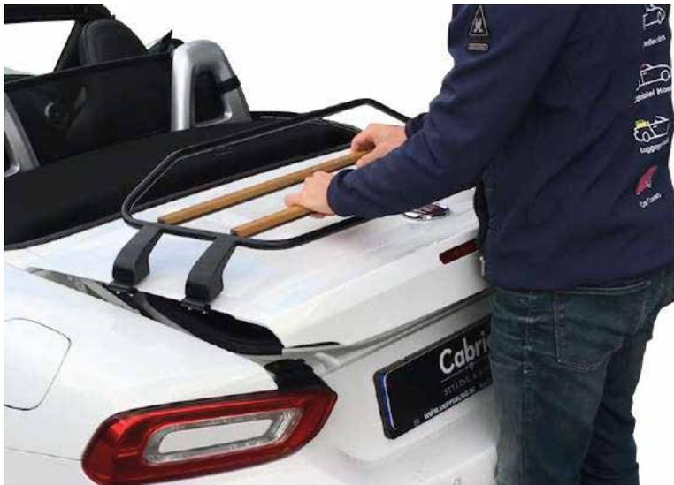
1. Loosen the side brackets with an inbus tool.
